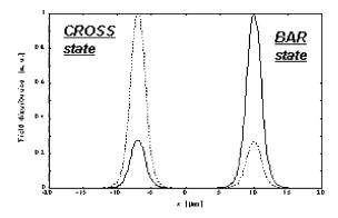
FIGURE 4 Field distribution on the output waveguides in cross state (dashed line) and in bar state (solid line).
