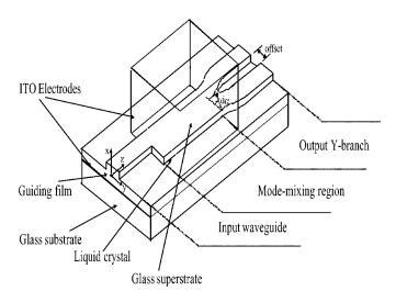
FIGURE 1 Schematic top view of the device.
